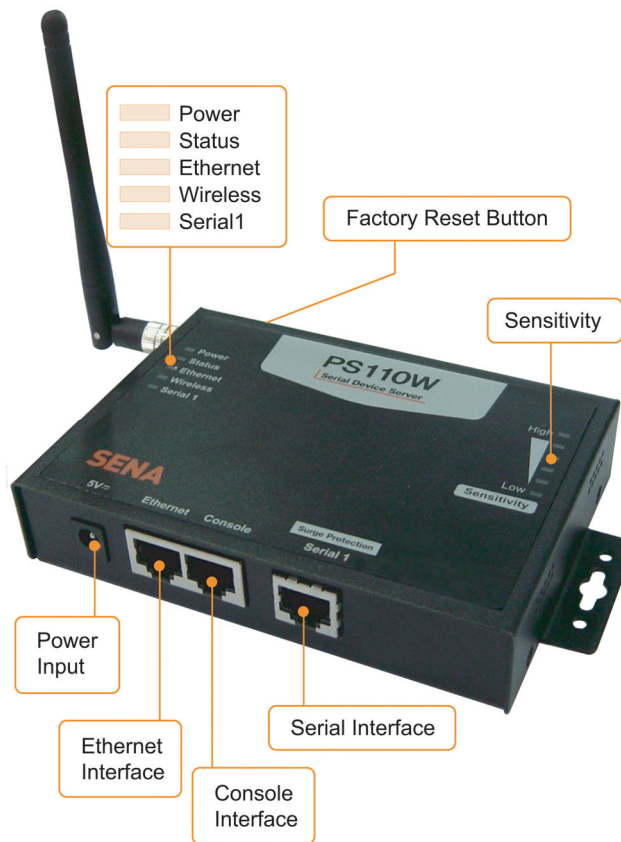
Figure 2-1 The panel layout of the PS110W
