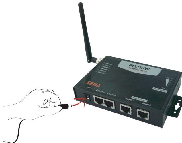
Figure 2-5 Connecting the power to the PSx10W
